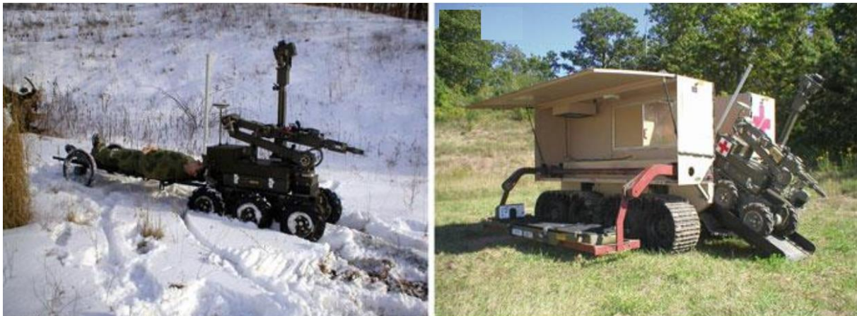
Figure no. 6: Robot extraction (REX) transporting the immobilized victim on a sled and (b) Robot Extraction (REX) and REV (robotic evacuation vehicle) 26
