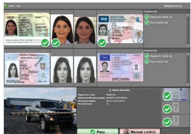
Figure no. 1: FastPass pilot system screen for the border guard to biometric identification of passengers arriving by passenger car 20
