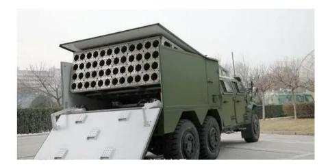
**Figure nr. 7**: The "Hummer" – type vehicle with 48 UAV launching tubes (Source: https://youtu.be/QamGaDNczJw)
